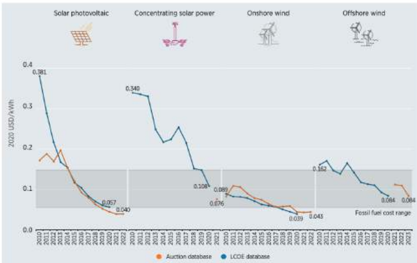
Figure ES.3 The global weighted-average LCOE and PPA/auction prices for solar PV, onshore wind, offshore wind and CSP, 2010-2023
